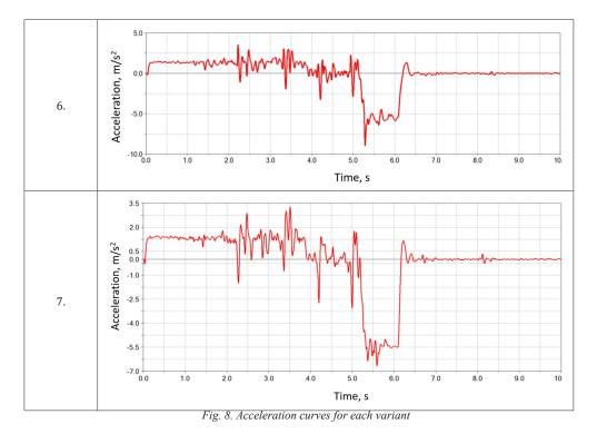
monorail. Fig. 8 shows the acceleration curves of the transport set in each simulation variant. Maximum and minimum accelerations for each of the analysed variants are shown in Fig. 9.
