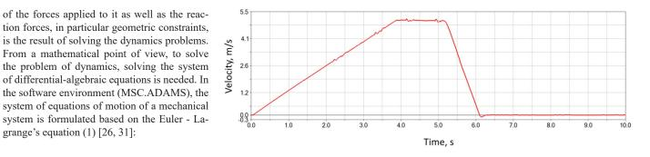
Fig. 7. The course of travel speed of suspended monorail unit in the MBS simulation
