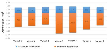
Fig. 9. Maximum and minimum accelerations for each of the analysed variants
